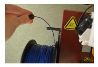
And just to be on the safe side, add the plastic guiding tube as well before you put the filament into the extruder:
