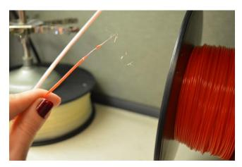
Clip that off (it can gum up the works if you try to reuse it next time) and pull the filament out of the plastic guiding tube.
