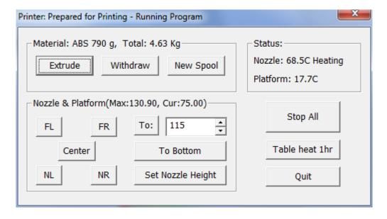
The nozzle will heat up again and start extruding the new filament. In the process, it will also push out the old filament. This is important for it to do in order to get a clean print, and it also looks very cool:
