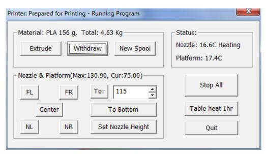
In this example, you'll see that we had a spool of PLA on there and about 156g left. (See below for suggestions on how to keep track of your filament.) Click on the button that says "Withdraw", and you can watch the temperature of the nozzle go up as it prepares to kick back the filament. It'll ultimately heat up to over 250C, and then the extruder will go in reverse, kicking out your filament, which will look like this:
